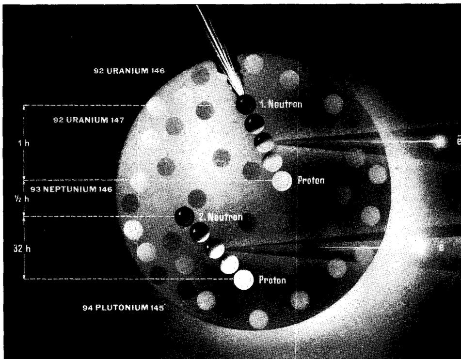
Fig. 43. THE TRANSFORMATION OF URANIUM INTO PLUTONIUM
